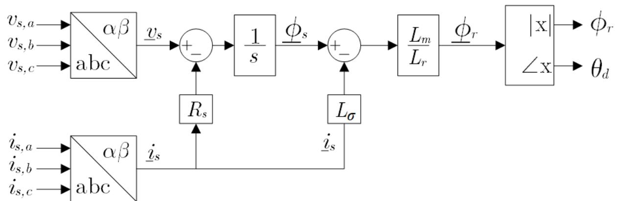
Then, the magnitude and the position of the rotor flux can be computed as:
